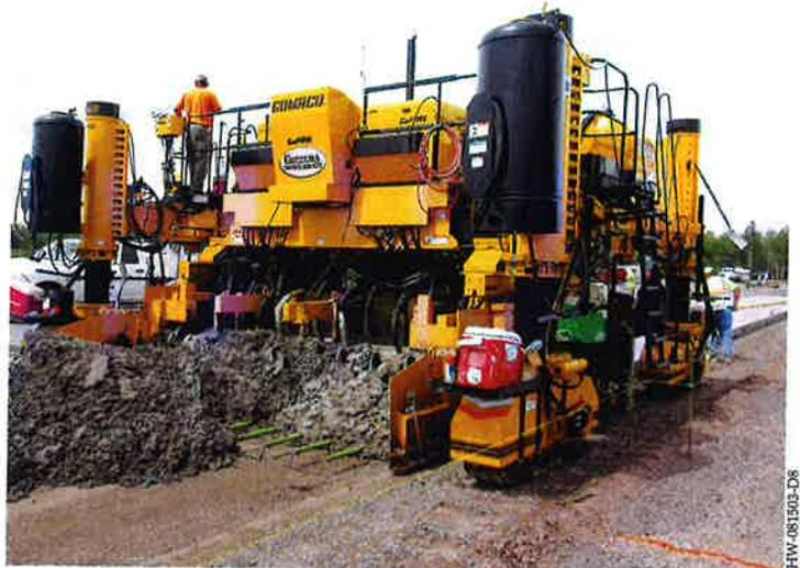
The Smart Width provides easy, accurate width change setup and also a reference for G+ to control proper steering and track speeds at varying widths of the paver.
